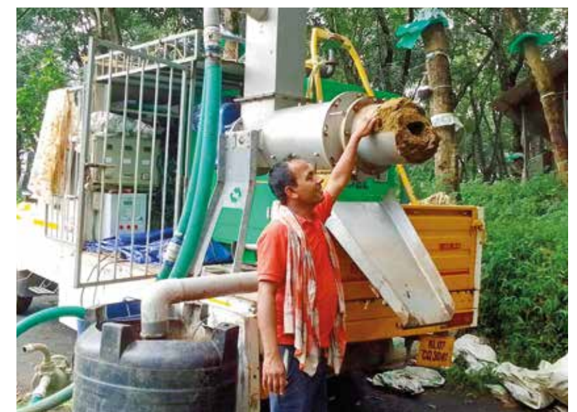
The machine dewateres cow dung from overflowing slurry pits
