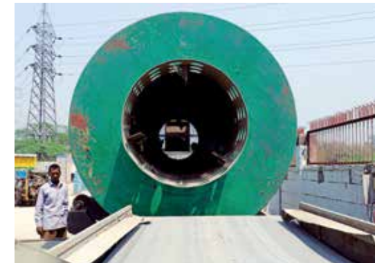
The drum rotates and separates dry and wet waste
