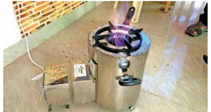
THE Applied Environmental Research Foundation (AERF) has developed a stove that uses agri-industrial waste for burning but doesn't emit smoke. It produces a clear blue flame. Named the My Forest Biomass Gasifier, the stove reduces indoor air pollution and saves forests.
