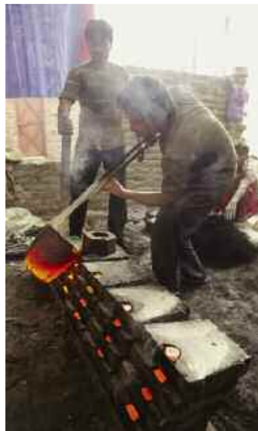
Molten brass being poured into a cast for handles
