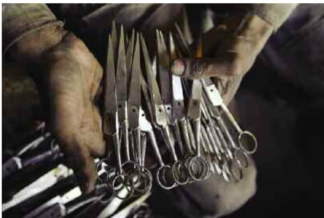
Barber scissors ready for riveting
