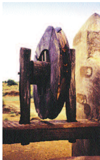
This rugged pulley is locally known as a Bhun. It is used to draw water from 300 feet.
