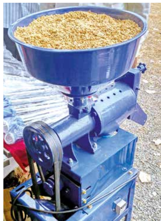
Paddy being hulled in the mini rice mill
